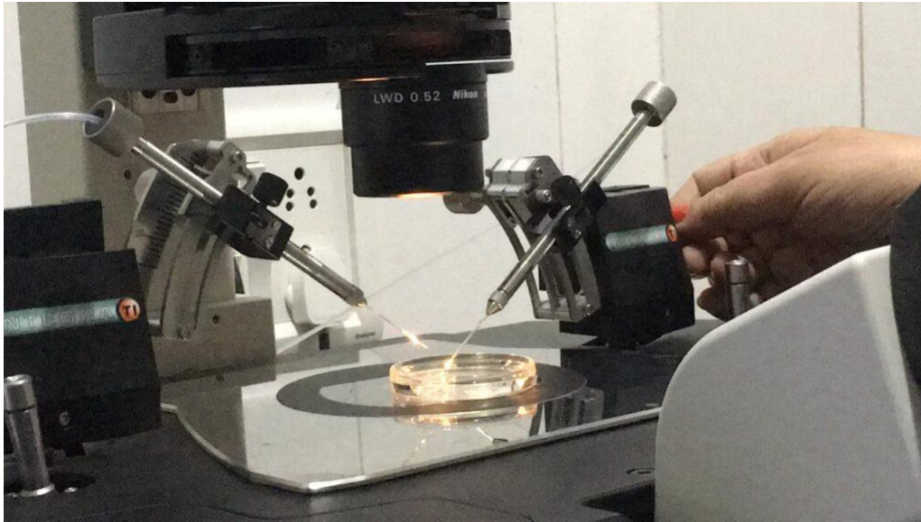
Holding Pipette(left) and Injecting Pipette(right) of the ICSI Micromanipulator. Petri Dish – Ovum and Sperm.
